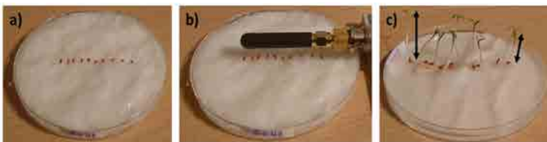
Figure 2: a) For each experiment, ten seeds of garden cress were placed next to each other onto water-soaked tissue layers. b) The helical antenna was placed directly above the cress seeds for applying the electromagnetic waves. c) After 100 h of germination and seedling the length of the cress seeds was measured.
