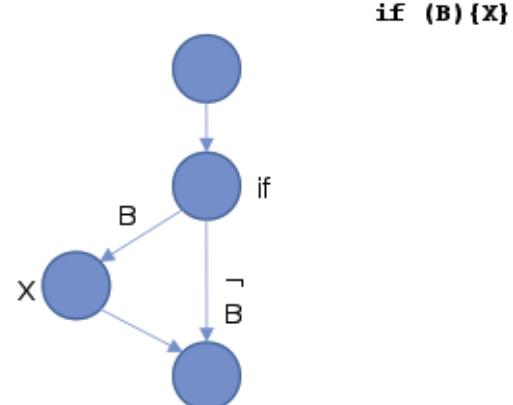
Figure 1: Example control flow graph for `if ( B ) { X; }`.
