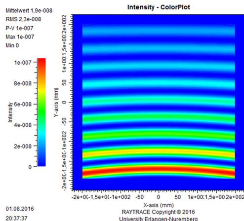
Figure 15: Distribution of the blue ( $\lambda_B = 450$  nm) component of reconstruction at the exit plane of the red ( $\lambda_R = 640$  nm) off-axis field lens (see Figure 13). The lower part represents the left display side.
