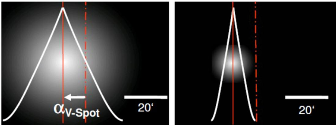
Figure 3: Image and Intensity distribution on an image sensor with  $\frac{1}{2}''$  CCD-camera and focal length  $f = 140/\text{F}\#5$
