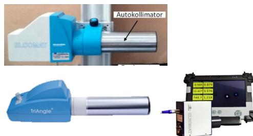
Figure 12: Instruments of electronic autocollimators for measurements DFR
