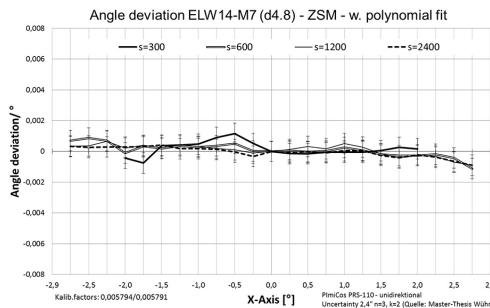
Figure 4: Result of the WiPoVi-Sensor calibration over a measurement range of  $\pm 2.8$  degrees at several distances from 300 to 2400mm. Error bars correspond to the uncertainty ( $k = 2$ ,  $1-\alpha = 95\%$ ) of the angular reference table PIImicos PRS-110.
