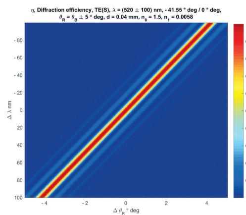
Figure 10: Calculated diffraction efficiency  $\eta(\Delta\theta_B, \Delta\lambda)$  of a Bragg diffraction based volume grating designed for a  $\lambda = 520 \text{ nm}$  anamorphic BLU geometry (10x in air).
