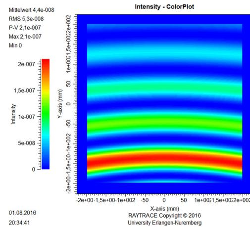
Figure 14: Distribution of the green ( $\lambda_G = 520$  nm) component of reconstruction at the exit plane of the red ( $\lambda_R = 640$  nm) off-axis field lens (see Figure 13). The lower part represents the left display side.
