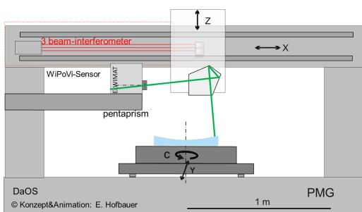
Figure 5. Setup of DaOS on Precision Measurement Granite portal PMG at Deggendorf Institute of Technology, shown in two edge positions. One of the emitted beam within the measurement range will always be perpendicular to the surface under Test SUT, and therefore will be reflected directly back to the sensor and will fit the aperture of the
