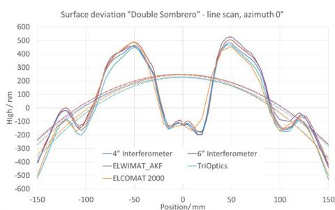
Figure 14: Interferometric and DFR measurements of plano-double-sombrero at azimuth 0°.
