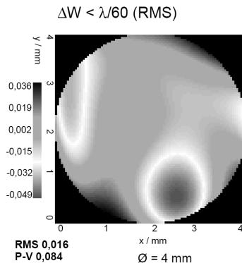
Figure 3: Measured wave front, diffracted by a volume grating (1<sup>st</sup> Bragg diffraction order [BDO], exit plane imaged onto the detector plane). The aberration is less than  $\lambda/60$ . The measurement area is equivalent to a representative area of the entrance pupil of the human eye EP ( $d_{EP} = 4$  mm).
