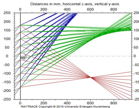
Figure 13: Top view of a Bragg diffraction based volume grating lens designed for  $\lambda_R = 640$  nm and  $10^\circ$  deg off-axis focus. The focal distance is 600 mm. The lens is illuminated off-axis with  $\lambda_G = 520$  nm,  $\lambda_B = 450$  nm and  $\lambda_R = 640$  nm. Illumination angles, which are reverse to diffractive dispersion, are used. The colors of the rays are equivalent to the wavelengths used.
