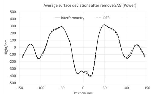
Figure 15: Averages of Interferometric and auto collimator DFR measurements at azimuth 0° after removing SAG error.
