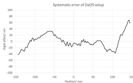
Figure 16: Evaluated systematic error of penta prism and V-SPOT sensor ELWIMAT 46-4,8 #19 by reverse measurement.
