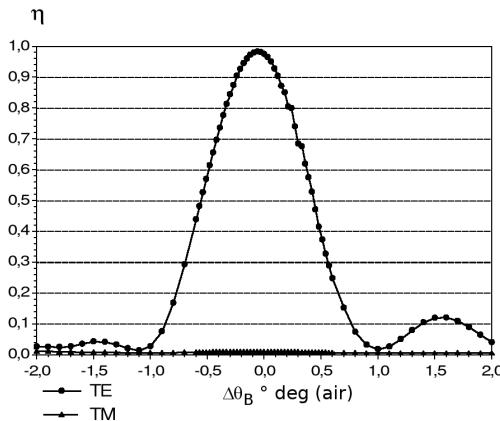
Figure 11: Measured angular selectivity of a Bragg diffraction based volume grating PBS illuminated with TE and TM polarized light. The diffraction efficiency is optimized for the second Bragg diffraction order (2<sup>nd</sup> BDO,  $\eta(\Delta\theta)$  in air). The grating period is  $\Lambda_2 = 600$  nm, the diffraction angle is 90 ° deg within  $n = 1.5$ . The design wavelength and the wavelength used for reconstruction is  $\lambda_R = 650$  nm.
