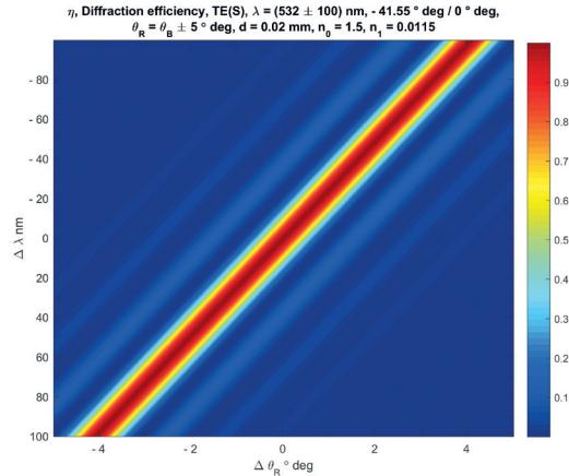
Figure 8: Calculated diffraction efficiency  $\eta(\Delta\theta_B, \Delta\lambda)$  of a Bragg diffraction based volume grating designed for a  $\lambda = 532 \text{ nm}$  BLU geometry.
