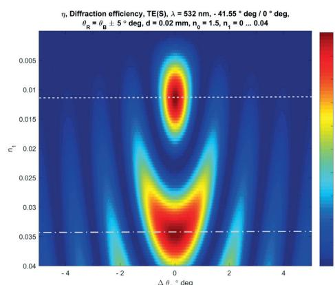
Figure 6: Calculated diffraction efficiency  $\eta(\Delta\theta_B, n_1)$  for an angular range of  $10^\circ \text{ deg}$  and refractive index modulation  $n_1$  of up to 0.04.
