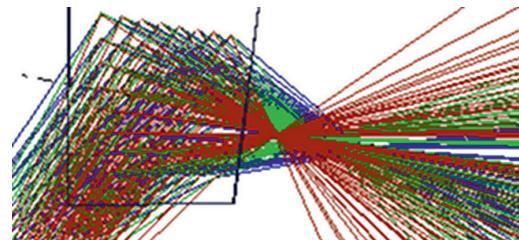
Figure 12: Raytracing of an off-axis Bragg diffraction based volume grating field lens, which is designed for  $\lambda_G = 520$  nm. The lens is illuminated with  $\lambda_G = 520$  nm,  $\lambda_B = 450$  nm and  $\lambda_R = 640$  nm wavelength. Collimated light enters the green off-axis field lens (comparable to VG2 in Figure 5) from the lower left-hand side. The lens is illuminated off-axis and forms an on-axis focus. The colors of the rays are equivalent to the wavelengths used.
