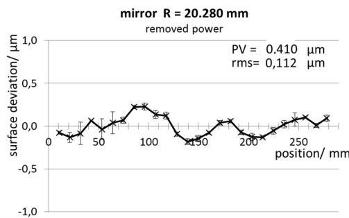
Figure 10: Surface deviation of mirror R 20.280 mm after correction of systematical errors by reversal measurement.
